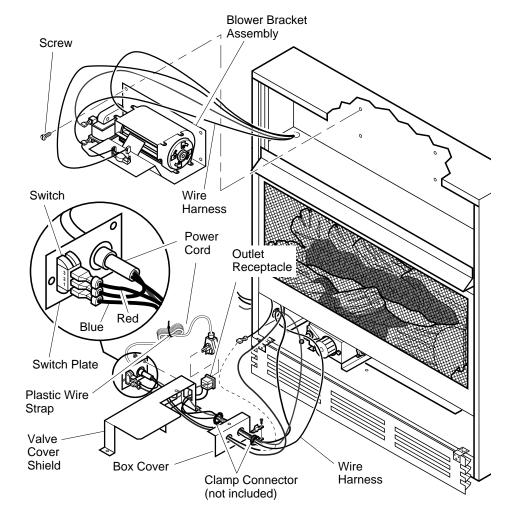
Figure 21 - Installing Blower Bracket Assembly
